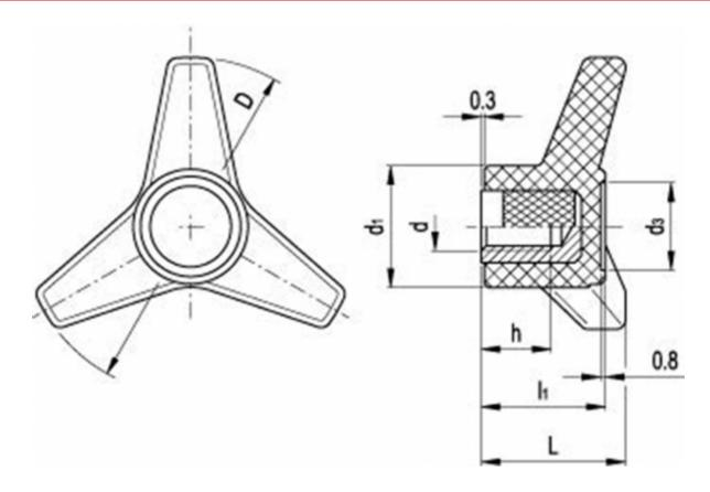
$\begin{array}{lll} D & = 100 \\ d1 & = 36 \\ d3 & = 25 \\ dh & = M12 \\ h & = 20 \\ l1 & = 36 \\ L & = 42 \\ Weight in (g) = 97 \end{array}$
